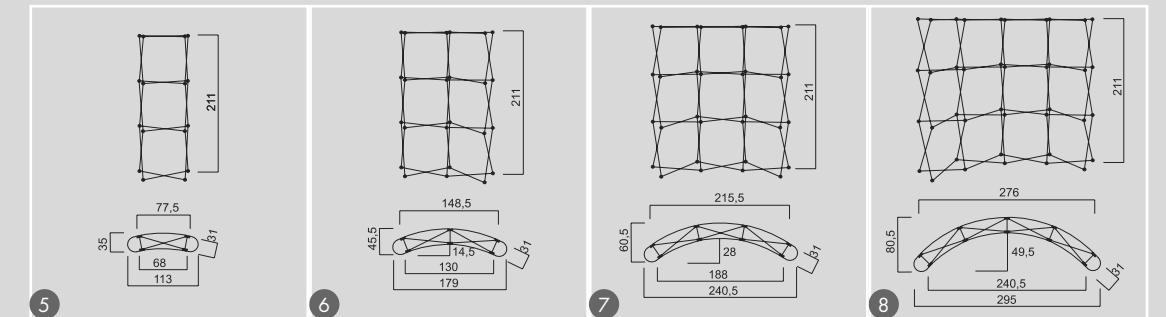
\*PARAMETERS MENTIONED IN THIS PART ARE DIMENSIONS OF THE STRUCTURES, NOT GRAPHIC PANELS
