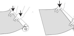
6.Return the roller with graphic into the base. LET THE ENTIRE GRAPHIC LAY OUTSIDE THE BASE. Close the cover.
